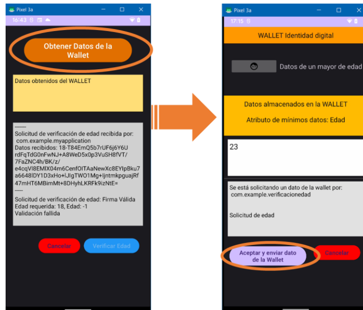
The age verification app receives the request from the browser and communicates with the digital wallet
