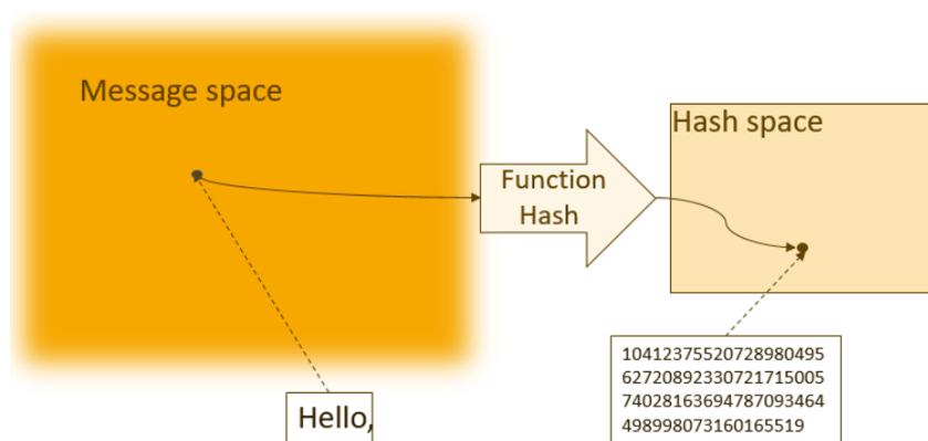
To the left, the message space is represented, that is, all possible datasets which may be created and from which a hash may be generated. In this figure, this set is represented with blurred limits, since this space may be infinite, given that it is always possible to create a larger message.
