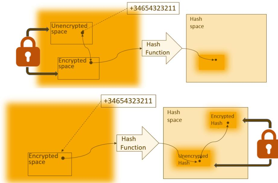
As shown in the figure above, encryption achieves a kind of correspondence between different message spaces, in the first instance, or, when the hash itself is encrypted, between two hash spaces.
