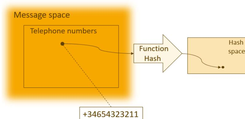
In the above figure, it is easy to see how the telephone number space is larger than the hash space. If all possible hashes for all possible 96 bits combinations were to be calculated, the entire hash space would inevitably be covered, and more than four thousand collisions would occur. In principle, the hash function would have to compress the 96 bits of the number into the 64 bits of the hash.
